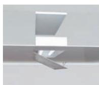
Clean room lighting fixture/luminary, sanitary type, 4x36 W; Light fittings constructed in 1 mm oven lacquered steel sheet to fit the sandwich type ceiling panel. Possible to inspect from both the top and the bottom (bottom part has no screws; it is fastened with internal springs). OSRAM electronic ballast included. Transparent diffuser (other diffusers available on request: Prismatic diffuser, opal diffuser or safety glass). IP54, CE mark.
